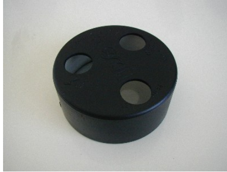
FIGURE 3.2. A Hartmann mask made from a 4" PVC endcap.
