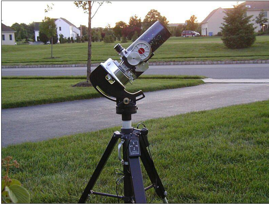
FIGURE 2.1. The 3.5" Questar telescope.
