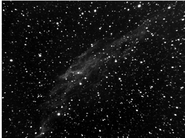
FIGURE 5.13. A calibrated image of the Veil nebula. Note the distorted star shapes around the edges and especially in the corners. This distortion results from an imperfect optical system. It becomes most evident when using a focal reducer.
